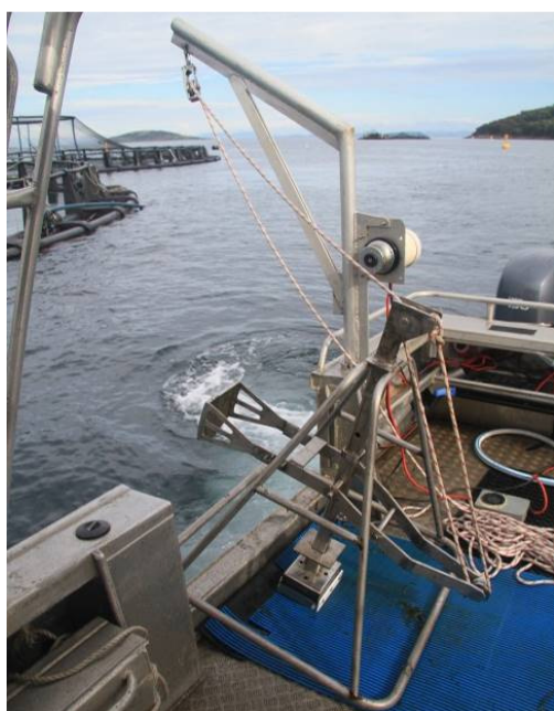
Figure 2-3 Multicore sampling device for mini cores (left) and an individual core sealed with latex bungs (right) used for metals sampling.
