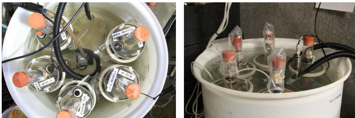
Figure 2-7 Mesocosm cores equilibrating with spacers under lids (left) and sealed and submerged during incubation (right).
