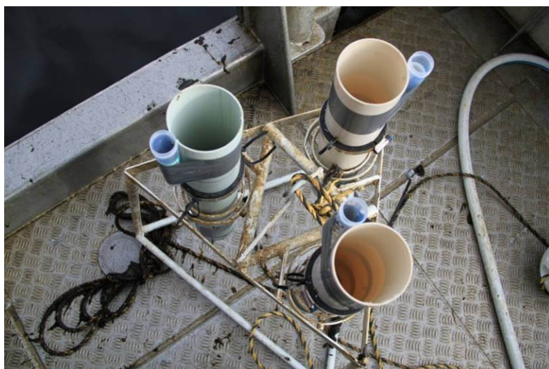
Figure 2-10 Sediment traps (note: 50ml container attached to the side of each core for collection of metal samples)
