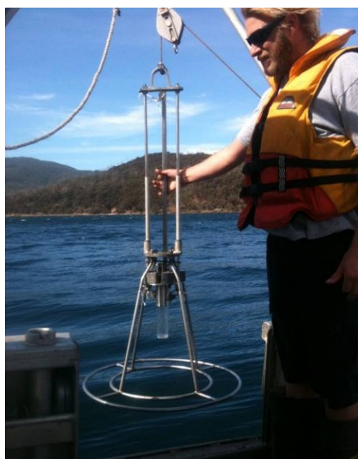
Figure 2-3 Multicore sampling device for mini cores (left) and an individual core sealed with latex bungs (right) used for metals sampling.
