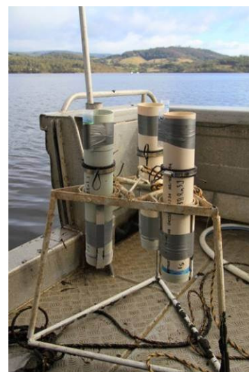
Figure 2-10 Sediment traps (note: 50ml container attached to the side of each core for collection of metal samples)
