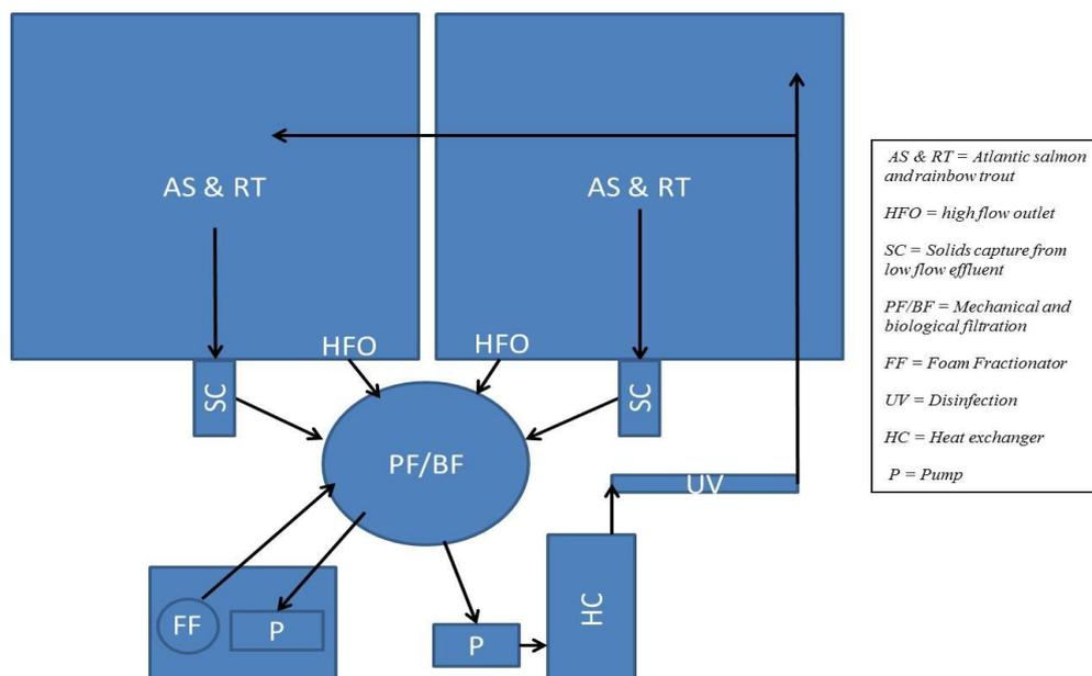
Figure 5. Modified recirculating system configuration used for housing mullet and Atlantic salmon during Experiment 6.
