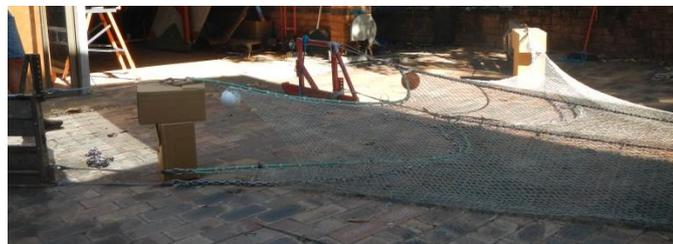
Fig. 3.9 Sweep lengths being tuned for proper trawl geometry
