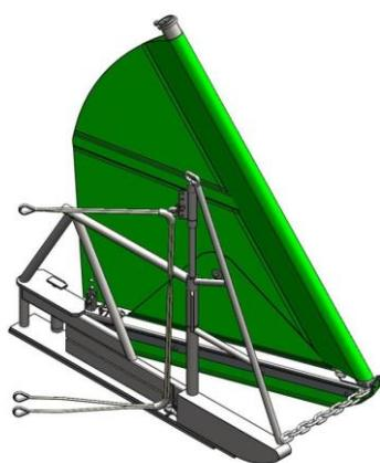
Fig. 4.2 Batwing otter board
