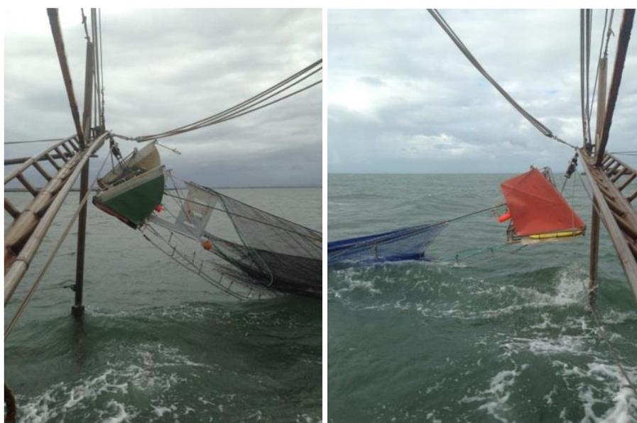
Fig. 4.4 Gear ready for shooting away at the end of the booms: 'W' trawl on the starboard and Florida flyer on the port side
