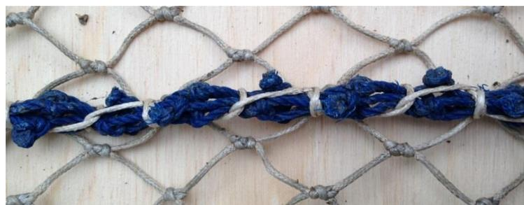
Fig. 3.4 Stretched netting sewn down the centre line with a hanging ratio of 0.707
