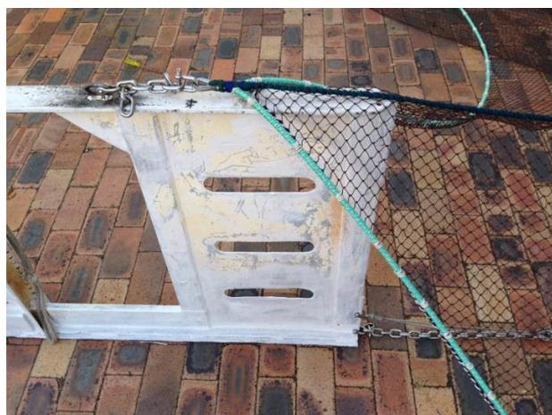
Fig. 4.3 Sled rigging
