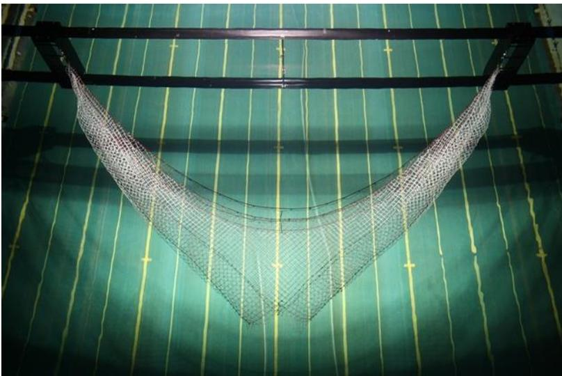
Fig. 2.5 Two model trawls (A on top and B on bottom) attached to the Trawl Evaluation Rig in the middle section of the flume tank
