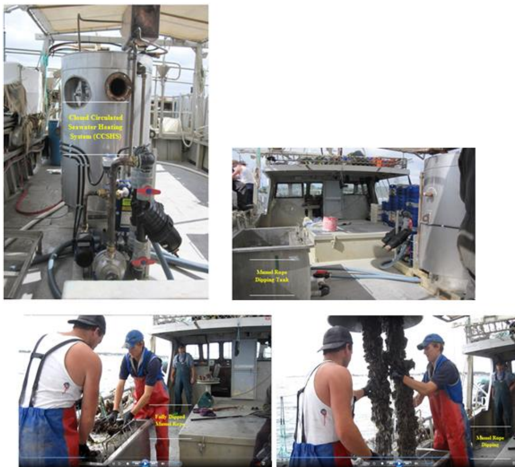
Figure 29: Offshore thermal treatment of the mussel droppers using “closed circulated seawater heating system (CCSHS)” machinery
