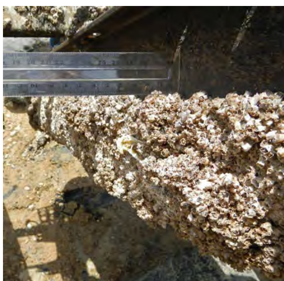
Figure 13. Multi-layered, stacked, barnacles on the side surface of a paddlewheel float. Colony depths up to 40mm were observed in this trial. Ruler included for scale.
