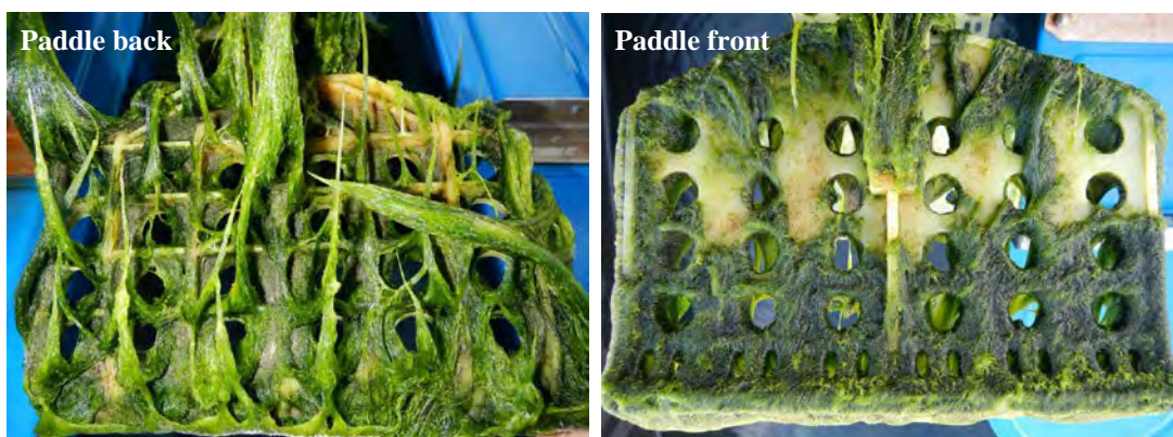
Figure 9. Blades of Futi 2hp paddlewheel tested. Paddles assembly removed from a fouled unit and placed on a clean one to provide data specifically for paddle fouling impact. Rotors combined wet weight of algae in air = 10.5kg.
