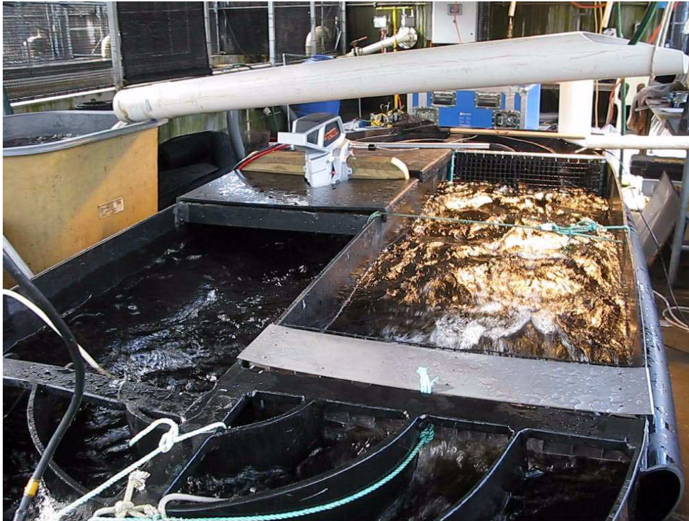
Figure 3.1: Freshwater swim trial at Saltas Wayatinah showing electric outboard (left side of picture) and fish challenge section with downstream collection screen (right side)
