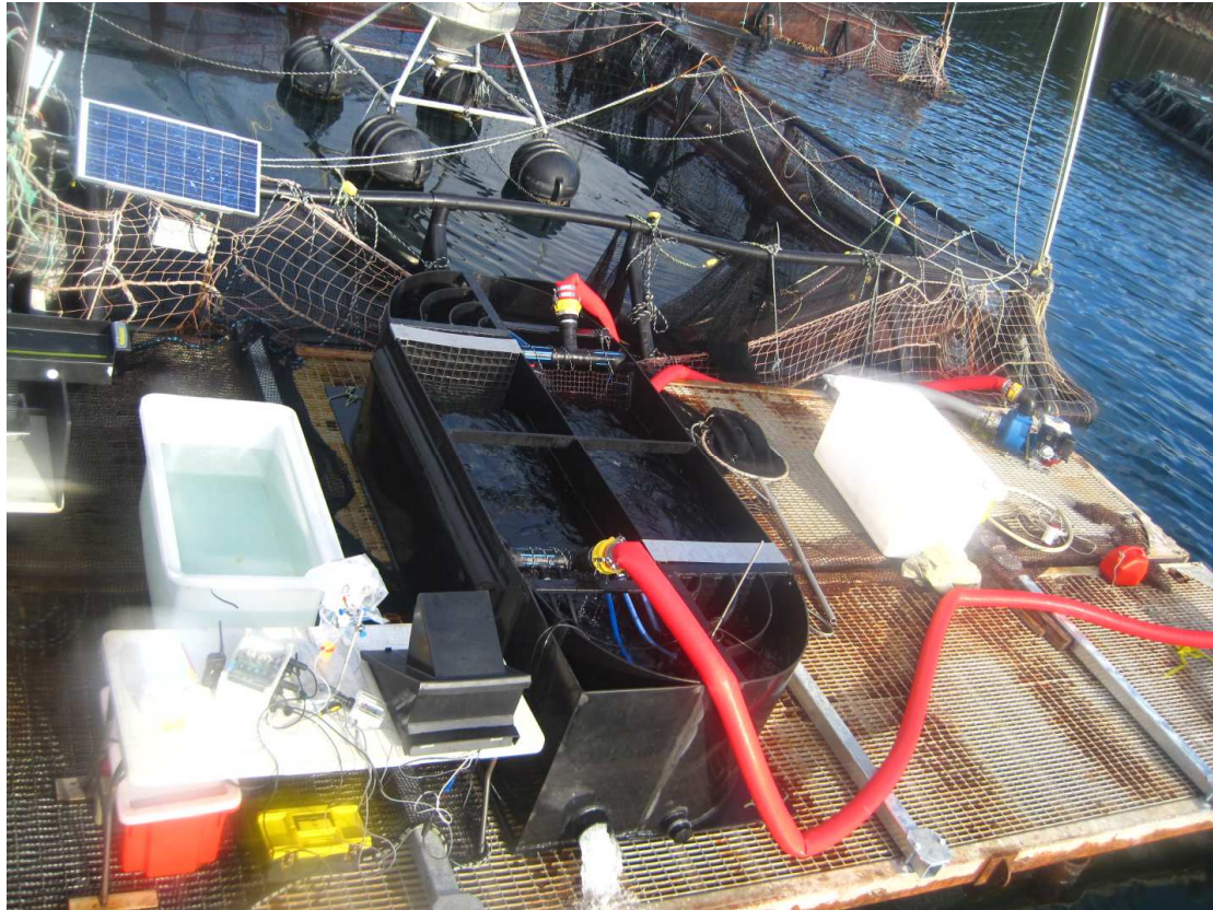
Figure 2.1: Layout of swim trial on floating pontoon, showing fish cage with jump fence lowered to transfer fish. Water is pumped to circulate water at velocity through two straight fish-challenge sections. PIT tag ID and time to fatigue is recorded before fish are placed in anaesthetic bath for measurement.
