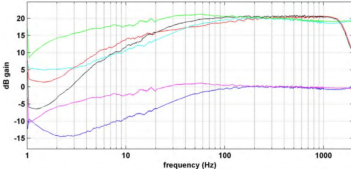
Figure 2. Sample sea noise logger system gain (pre-amp and recording system) showing frequency from the 2015 experiment: red - 3389, 20 dB system gain; black - 3300, 20 dB gain; blue - 3391, 0 dB gain; cyan - 3391, 20 dB gain; green - 3392, 20 dB gain; magenta - 3392, 0 dB gain. The curves were used over the frequency range above 5 Hz.
