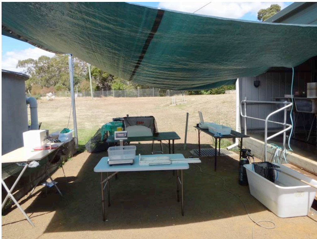
Figure 1. Makeshift out-door surgery theatre. In the foreground are anaesthetic setup fitted with aeration (right) and the measuring table (middle). In the rear are the portable ultrasound setup (right) and the surgery table (middle) with plastic bin (labelled carp) fitted with cradle (with black net skirting) to hold fish during surgery.
