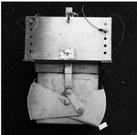
Figure 3-2 Box core (left) and Perspex liner used for sediment sampling.
