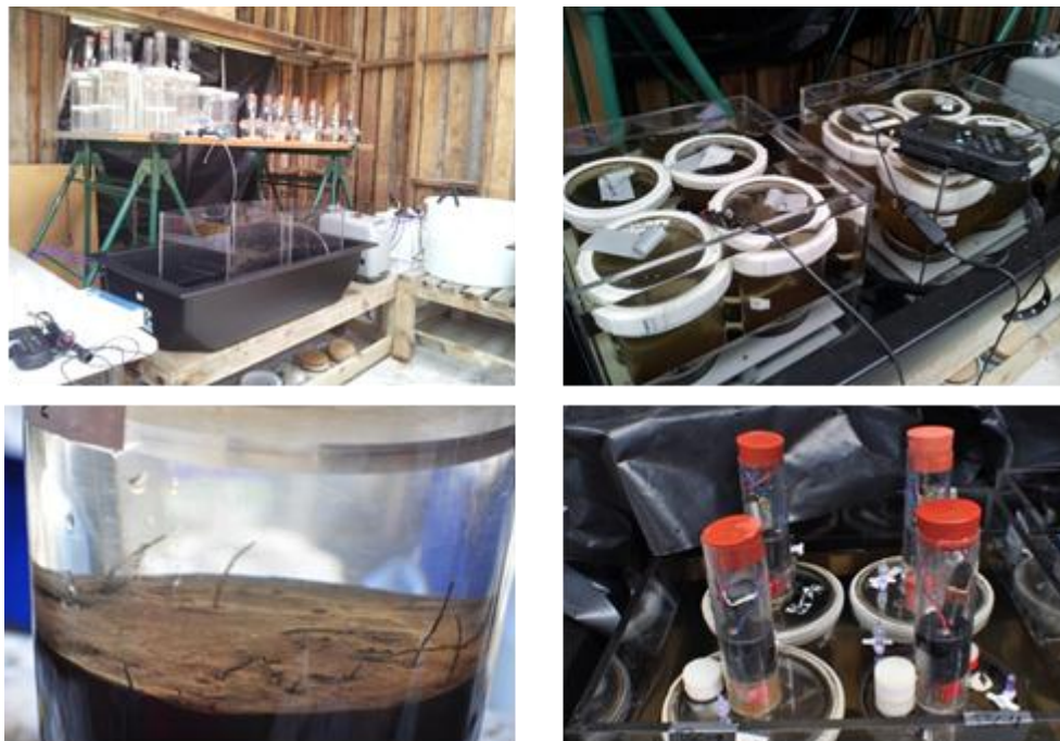
Figure 3-4 Pictures of lab set up (top left) - the large black tub acts a temperature control bath with circulating freshwater connected to the heater/chiller units, the clear Perspex aquaria hold the mesocosm and are filled with site bottom water (top right). The picture on the bottom left shows a close up of the sediment surface with faunal tubes and the picture on the bottom right shows the mesocosms with stirrer lids attached.
