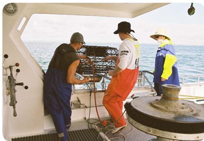
Using a winch and pot tipper makes for safe and efficient fishing operations.
