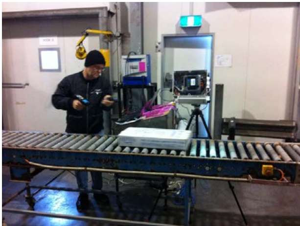
Figure 12 RFID and barcode scanning of labelled cartons at Doboy Cold Stores
