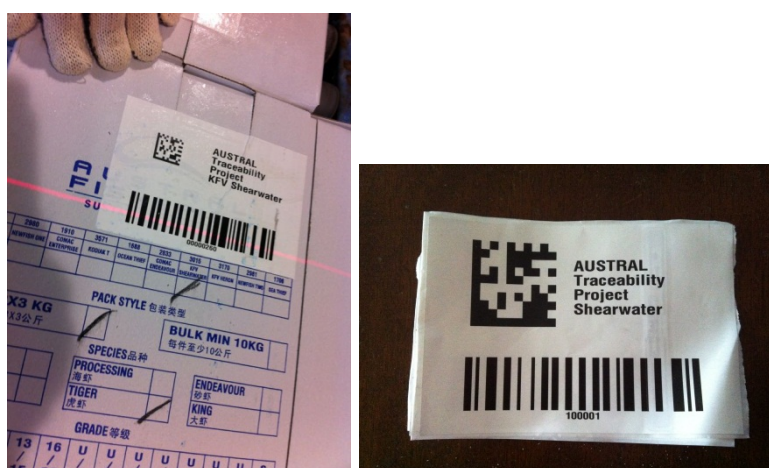
Figure 9 Carton label with 1-D and 2-D barcodes and RFID tag
