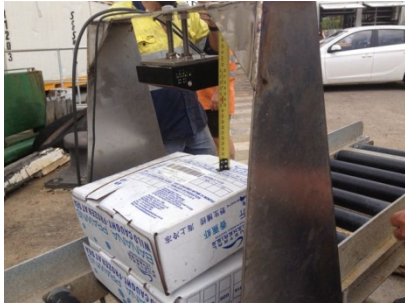
Figure 8 Labels and conveyor system with fixed scanner for Trial 1 on the 'Shearwater'
