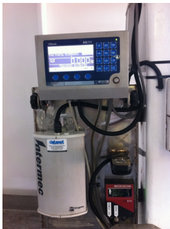
Figure 10 1-D, 2-D and RFID scanners installed on 'Shearwater'
