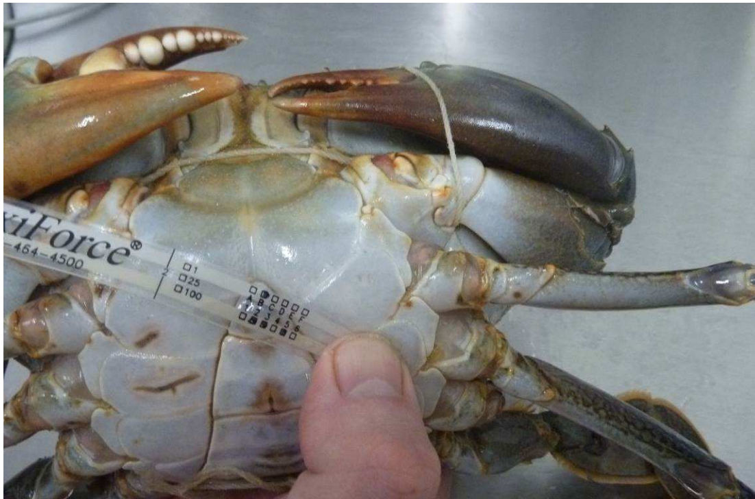
Plate 3.7 FlexiForce sensor used to measure pressure of shell flex.
