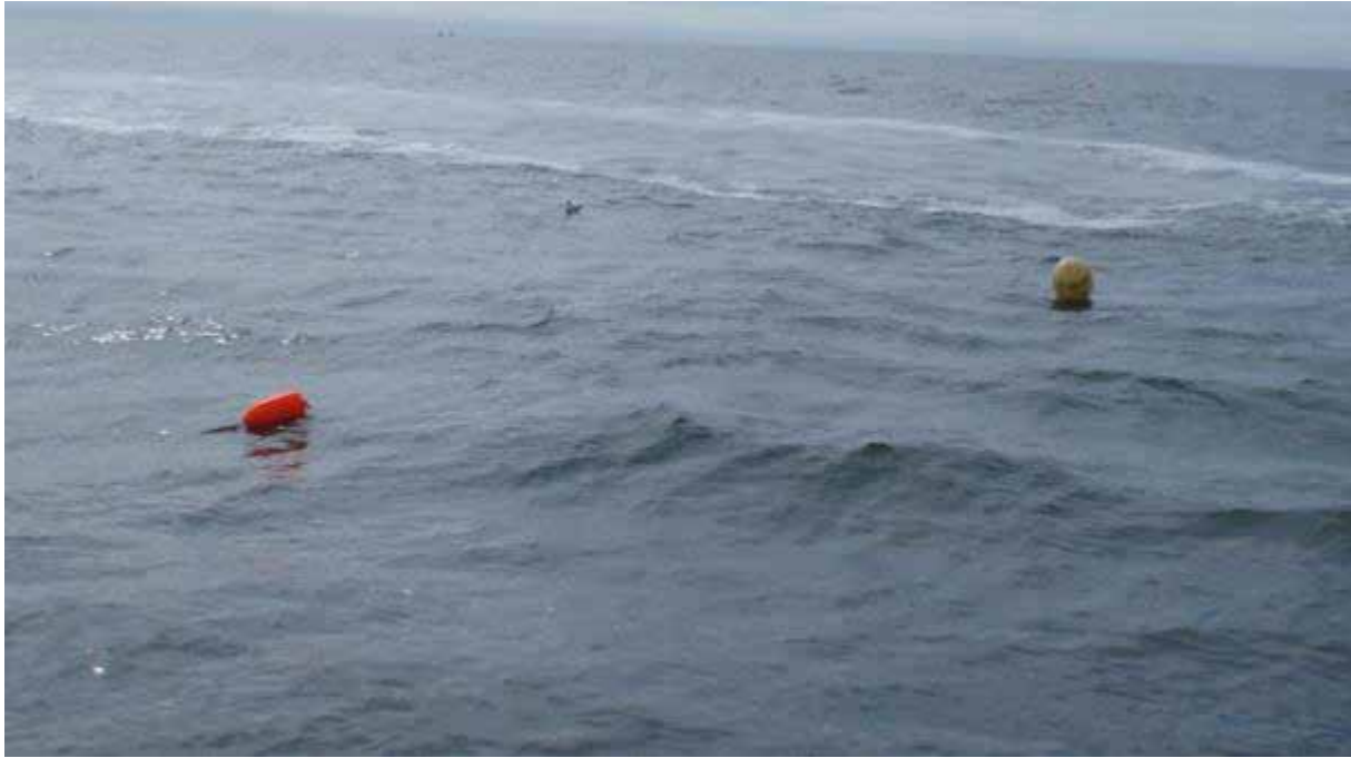
Plate 3 Float rig used in Cutler (NE Maine) showing the two buoy system used due to the strong current conditions. There is no floating line between the buoys
