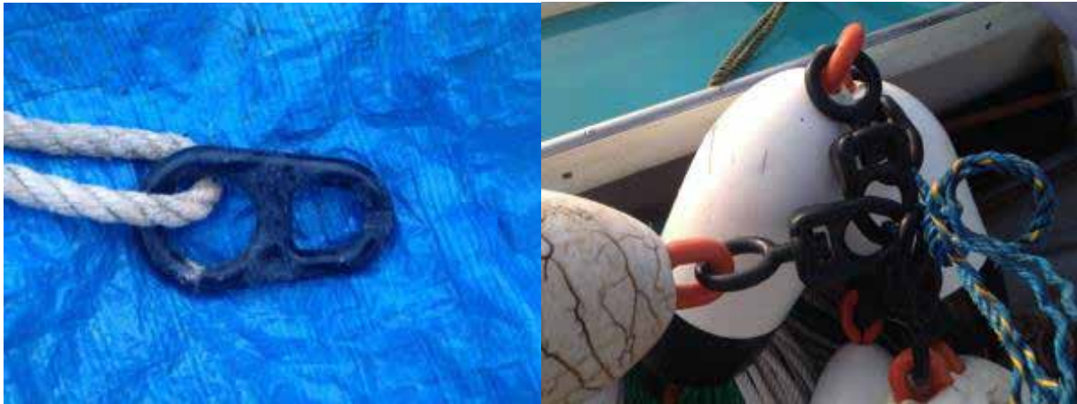
Plate 1 Two different types of weak links used in the Maine Lobster Fishery
