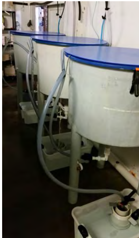
Fig. A3.3. 300 L cylindro-conical fibreglass spawning tanks complete with the egg collection screens.
