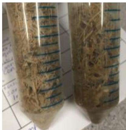
Figure 13 Samples with 1:3 acid to bone ratio without water ( left) and with water (right) after 24 hours.
