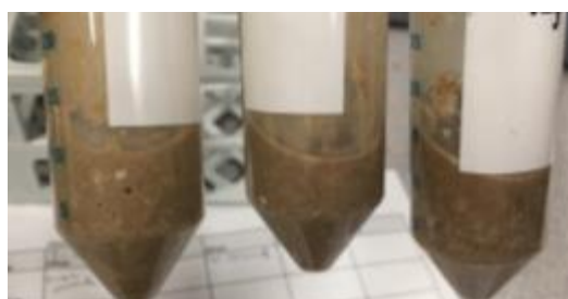
Figure 14 Treatments with 2:1, 3:1 and 4:1 acid to bone after 24 hours digestion and agitation.
