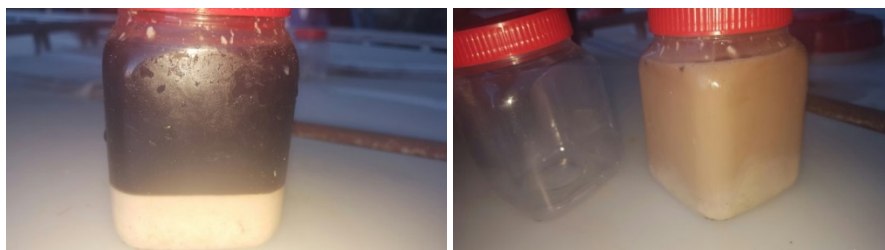
Figure 13 Factory trials with bones in phosphoric acid: A: not shaken, and B: shaken.
