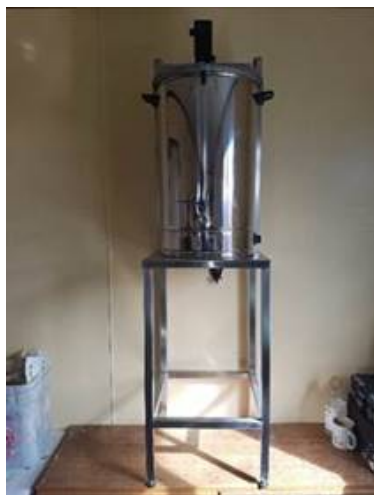
Figure 5 40L experimental hydrolysis unit
