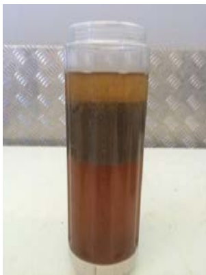
Figure 9 Patagonian Toothfish hydrolysis fractions following sitting for 24 hours
