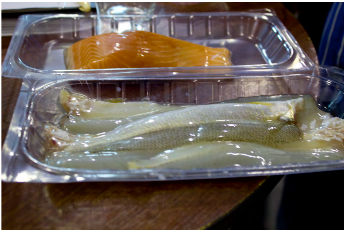
Figure 3: Photograph of packaged finfish. These packets are thermoformed with a top film draped across the product forming a tight vacuum.
