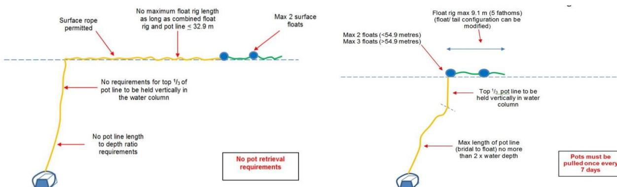
Figure 2 Diagrammatic representation of the gear modifications required in a) shallow (~<20 m) and b) deep (~>20 m) water depth
