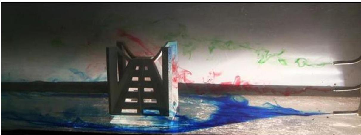
**Figure 61:** Artificial reef module being tested in a university flume tank (Subcon Pty Ltd).
