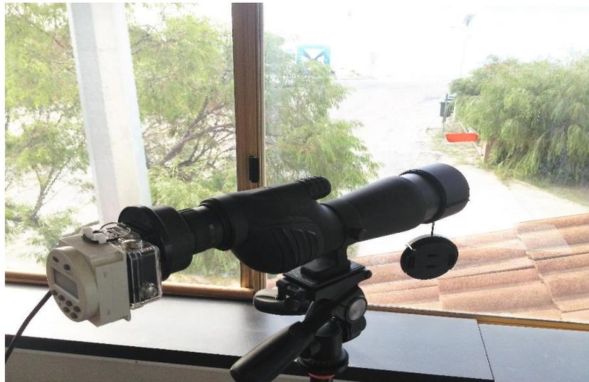
**Figure 35:** GoPro Hero4 Camera attached via lens adaptors to a Redfield 'Rampage' 20-60x60mm Spotting Scope. The CamDo Time Lapse Intervalometer can be seen 'piggy backed' onto the camera which was programmed to take three pictures, one minute apart.
