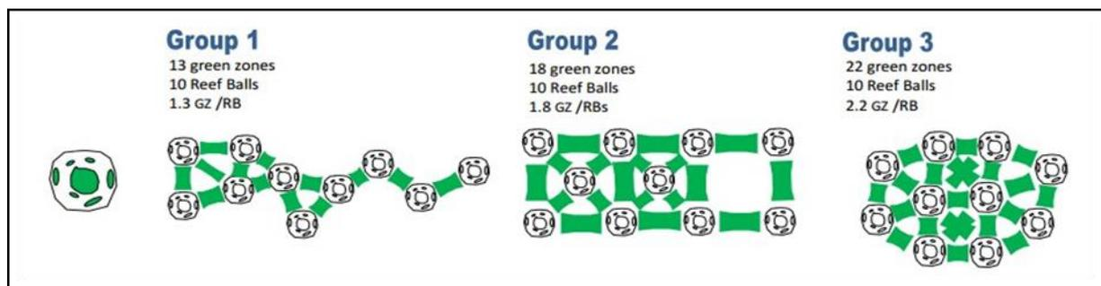
**Figure 62:** An example of interstitial spaces as 'Green zones' using Reef Ball™ modules (Lennon, 2011).
