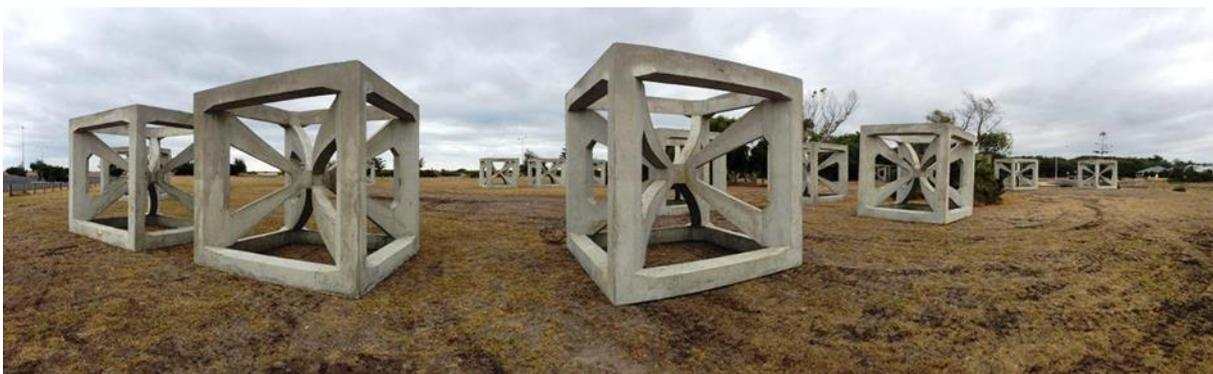
**Figure 56:** Concrete reef modules awaiting deployment.
