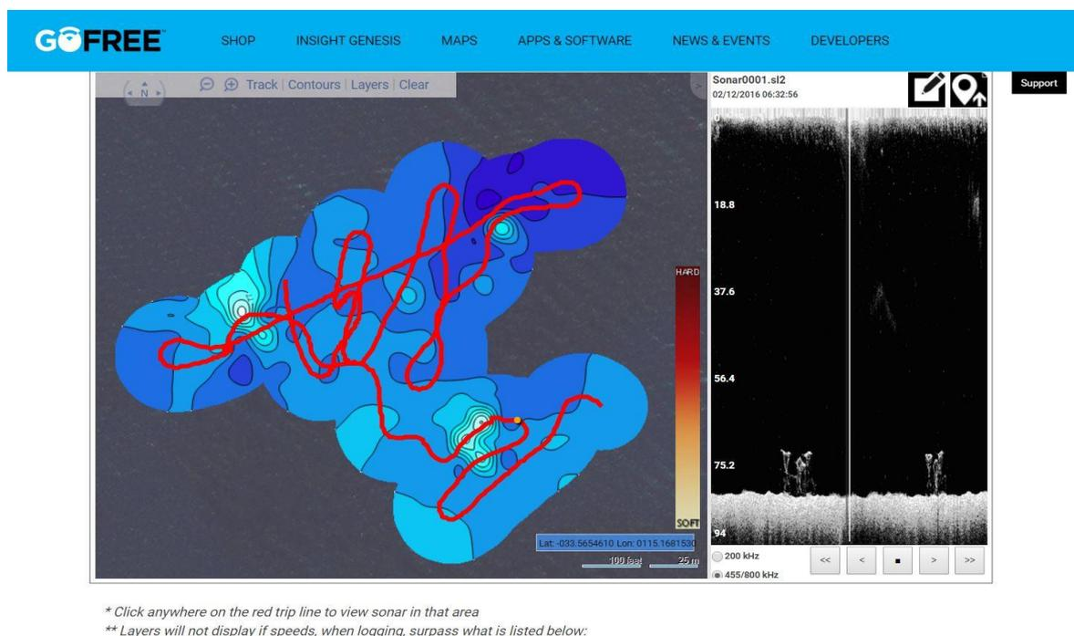
**Figure 38:** Sounder mapping details of Dunsborough Artificial Reef (note modules on right).
