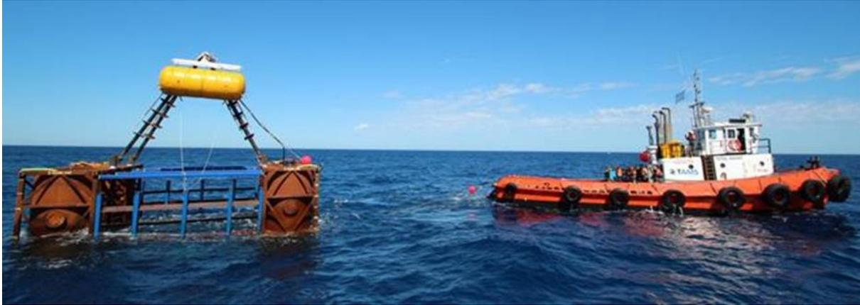
**Figure 67:** Tug boat towing a ‘Fish Tower<sup>TM</sup>’ module to its final deployment site.
