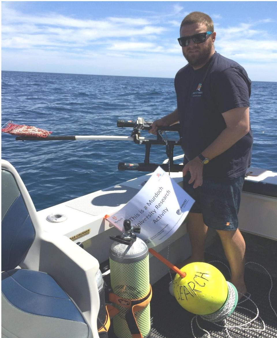
**Figure 25:** Reef Vision volunteer deploying a Baited Remote Underwater Video system.
