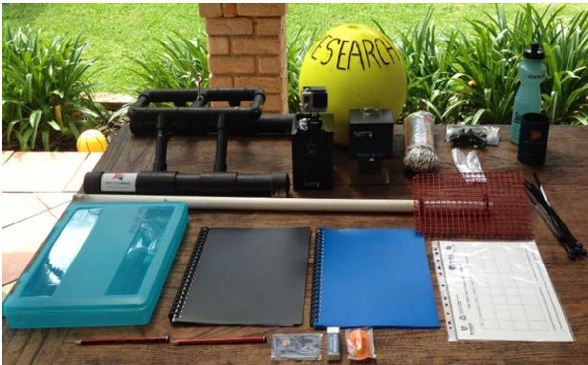
**Figure 41:** The package supplied to volunteers at the workshop including the BRUV unit, promotional material, data storage devices and metadata collection materials.
