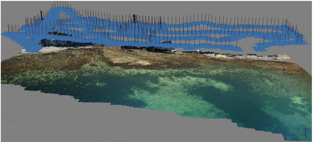
Figure 14: Perspective view 3D model and flight path
