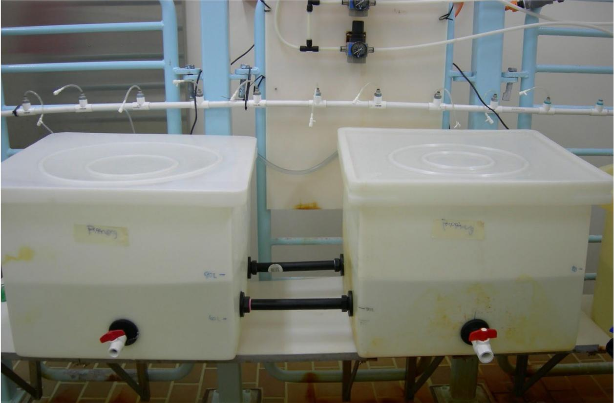
**Figure 10a: Square tanks joined by tubing, used to assess infection by co-habitation**
