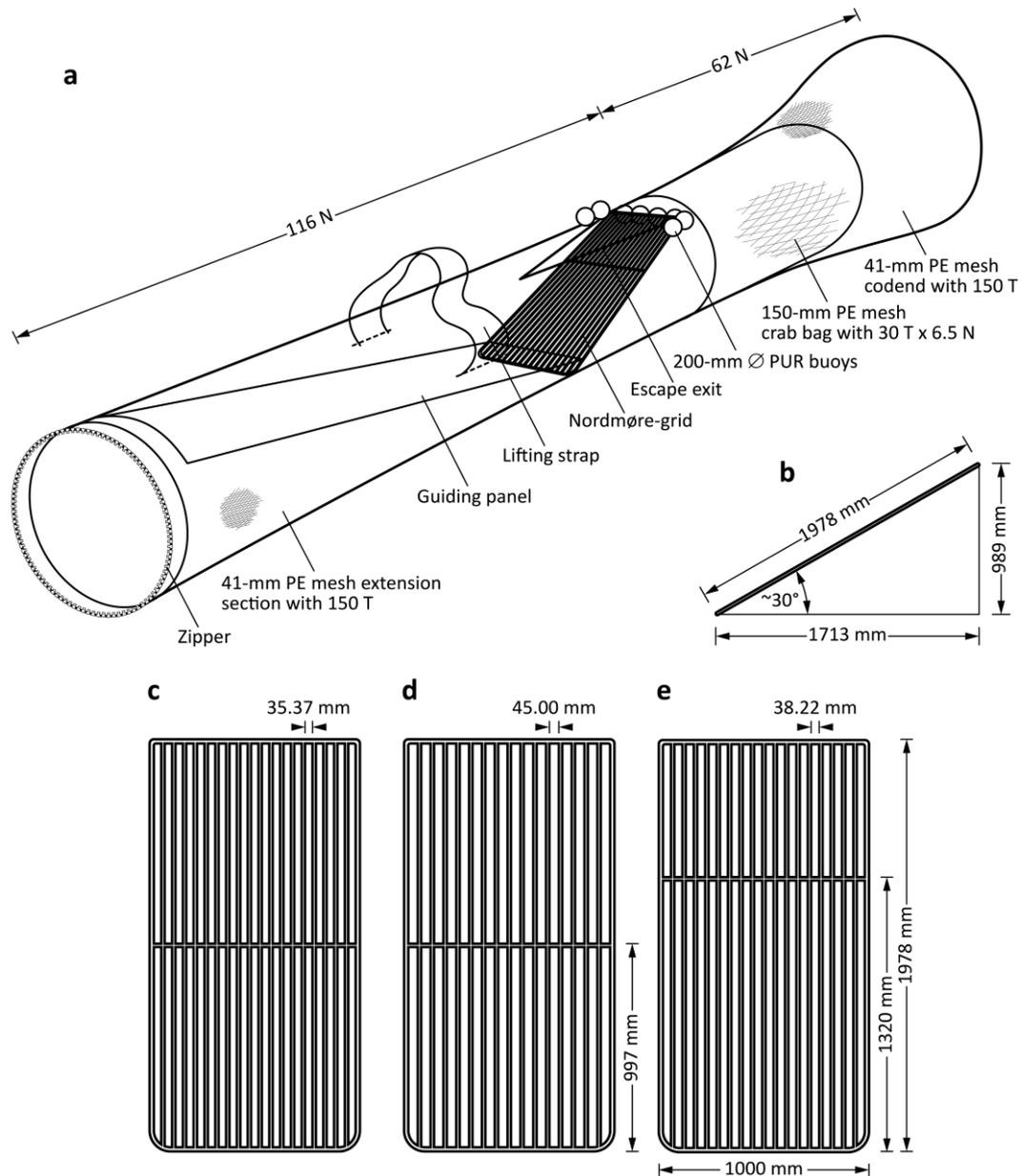
Fig. 3. Specifications of the (a) extension and codend (with crab bag) assembly with a Nordmøre-grid installed, (b) installation angle and (c) 35-, (d) 45- and (e) 38-mm grids tested. PE, polyethylene; PUR, polyurethane; T, transversals; N, normals; Ø, diameter.
