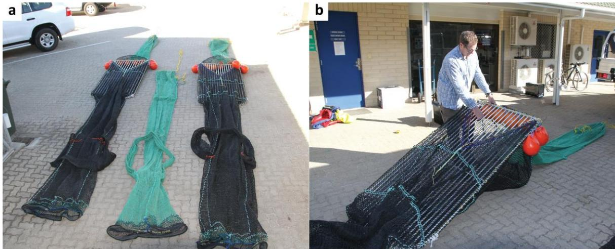
Fig. 4. The (a) 45-mm (left) and 35-mm (right) Nordmøre-grids and their extension sections/codends, either side of a control codend (centre), and (b) close-up of the 35-mm grid.
