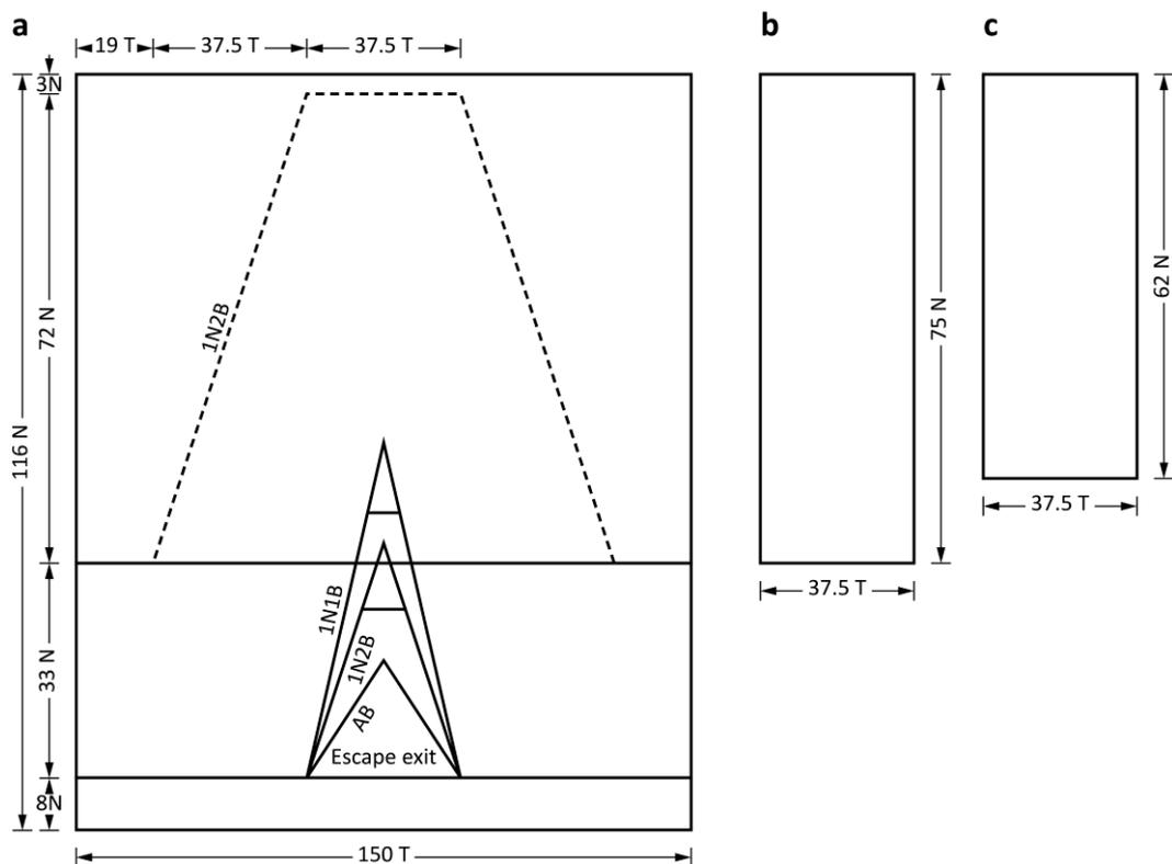
Fig. 5. Plans of the (a) extension cylinder showing the AB-, 1N2B- and 1N1B-exit openings, and (b) 75-N and (c) 62-N guiding panels. T, transversals; N, normal.
