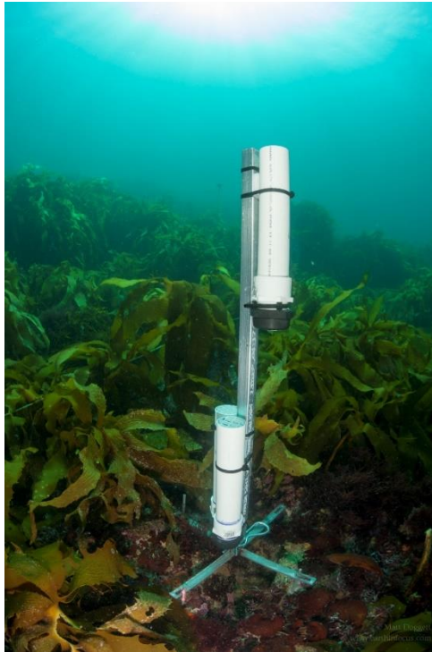
Figure 6.7-4 Sediment trap installed in reef habitat (Picture: Cayne Layton).
