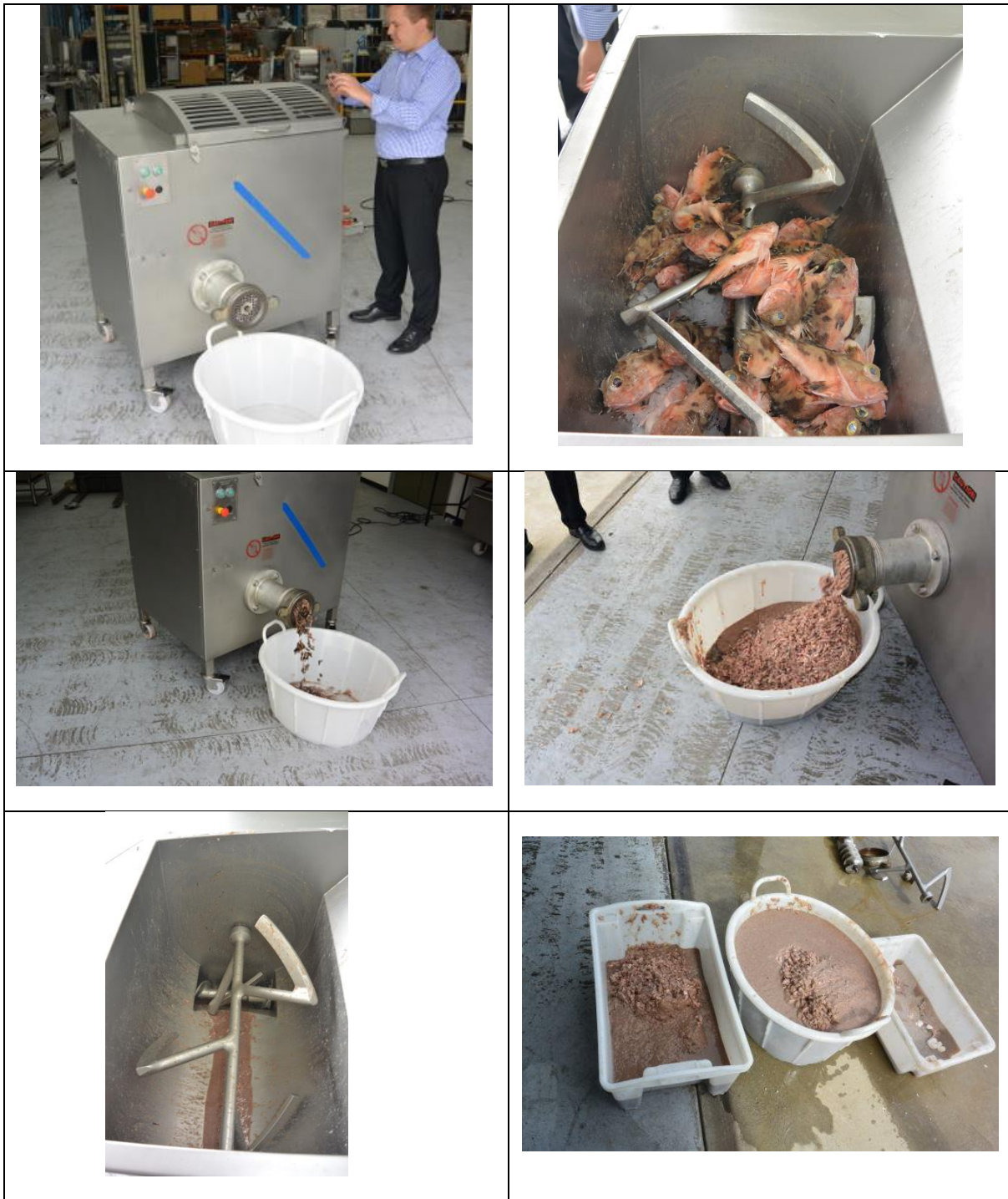
Figure 40. The Thomson 3000 Mixer/Mincer. Top right: with 25 kg of Thetis Fish. Middle left: Starting mincing through 10 mm plate. Middle right: Mincing through 10 mm plate. Bottom left: Residue left over after 75 kg of fish minced. Bottom right: Total output. The majority of the output is mince, however it is largely covered by sludge that was ejected near the end of each bin, and rose to the surface.
