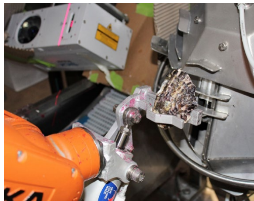
Figure 6. Robot picking up oyster from the carousel
