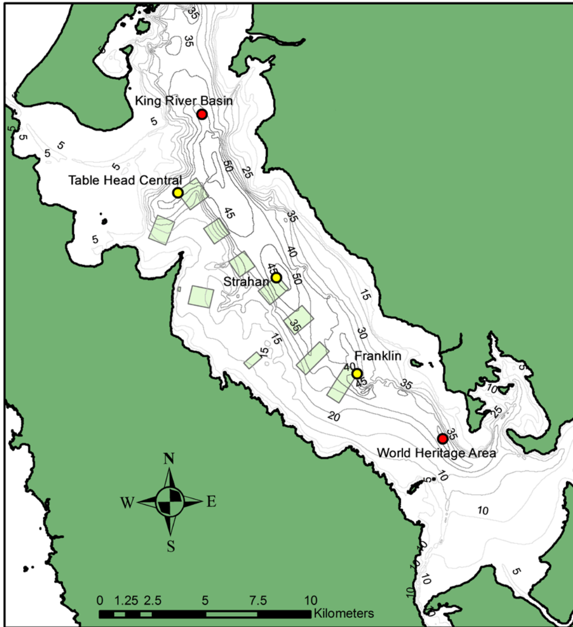
Figure 2 Map of Macquarie Harbour showing location of the environmental strings. The yellow sites provide data in near real time and the red sites use delayed mode data loggers. The CSIRO profiling mooring was directly adjacent to the Strahan environmental string until mid-2018 before it was moved to near the King River Basin site to help better capture the intrusion of oceanic water into the harbour.
