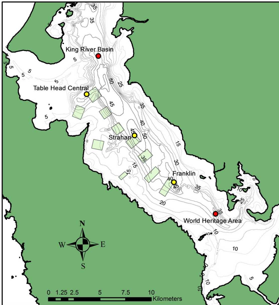
Figure 2 Map of Macquarie harbour showing location of the environmental strings. The yellow sites provide data in near real time and the red sites use delayed mode data loggers. The CSIRO profiling mooring is directly adjacent to the Strahan environmental string.
