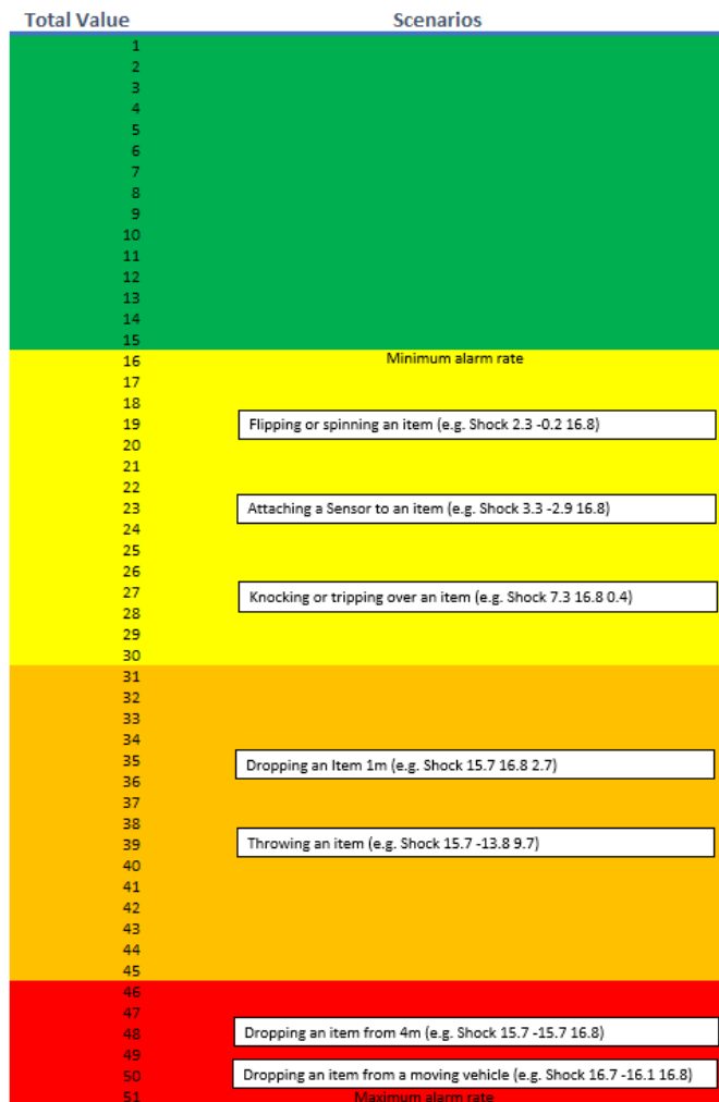
Figure 27 Testo G1 Sensor Shock Methodology Range
