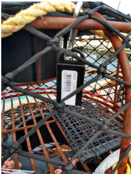
Figure 37 Scilex GPS pot tag attached to a lobster pot.
