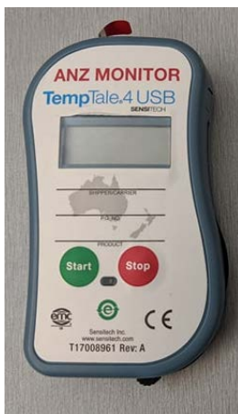
Figure 25 TempTale 4 USB Sensor
