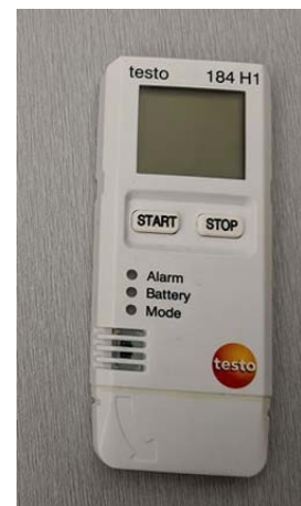
Figure 26 Testo H1 USB Sensor
