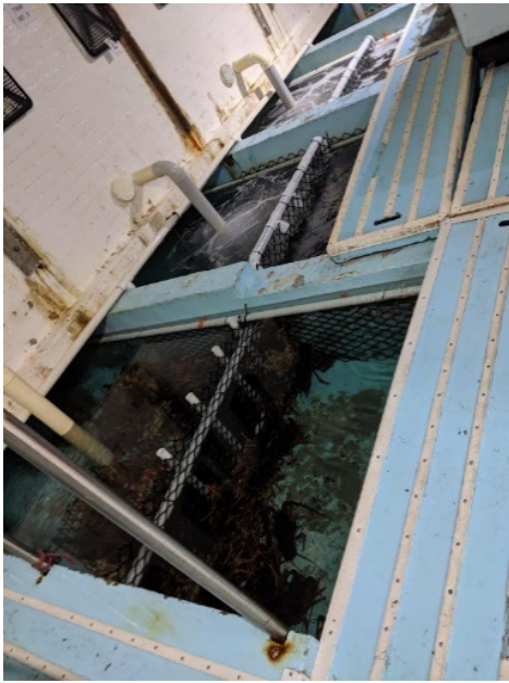
Figure 30 Installed tank separators for grade storage
