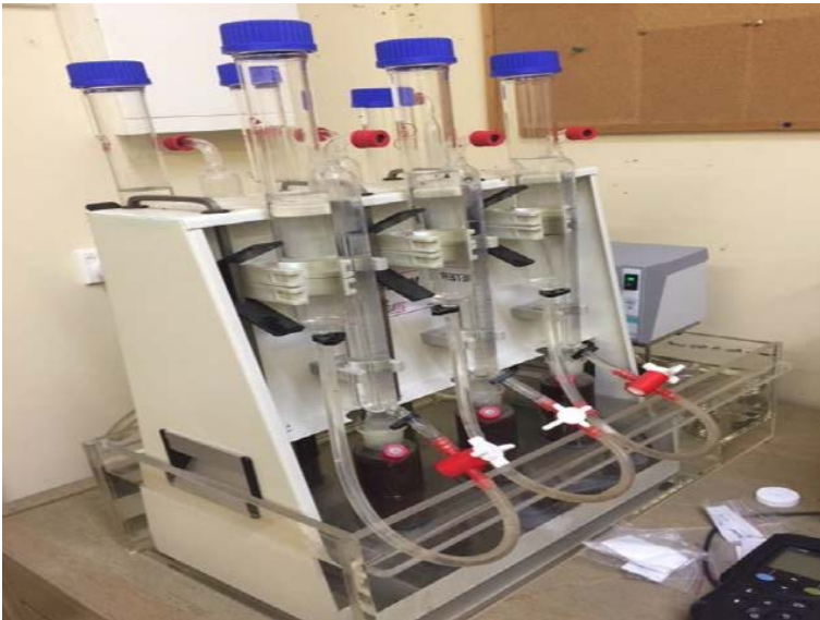
FIGURE 5: THE EXPERIMENTAL SETUP FOR THE ANAEROBIC DIGESTION TRIALS.
