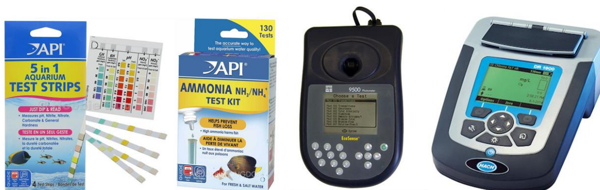
Figure 1: Test kits and photometers assessed for accuracy, ease of use and costs for water quality analysis.
