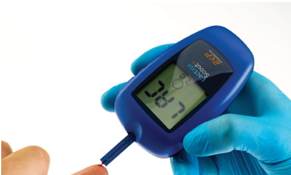
Figure 1. The Lactate Scout+ handheld meter examined in the present study for its effectiveness for the rapid and easy to use testing approach to quantify the concentration of lactate in Southern Rock Lobster haemolymph.
