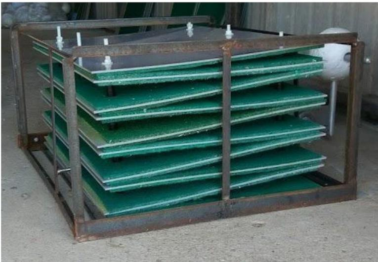
**Figure 55** A crevice collector trial as part of a pilot study.
