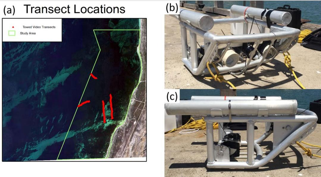
**Figure 35 (a) The location of the towed video transects used by this study. (b) oblique and (c) side view of the bottom tending towed video system used by this study.**
