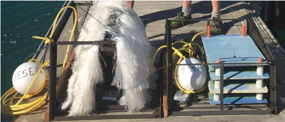
**Figure 54** Two prototype early juvenile lobster collectors, the benthic puerulus collector (left) and crevice collector (right) trialled as part of a pilot study.
