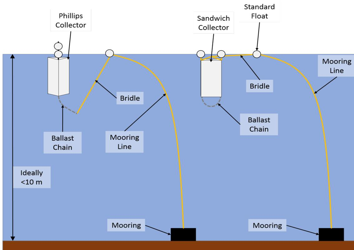
Figure 68 Typical puerulus collector deployment design for the "Phillips" type collector (shown left) and "sandwich" type collector (shown right).
