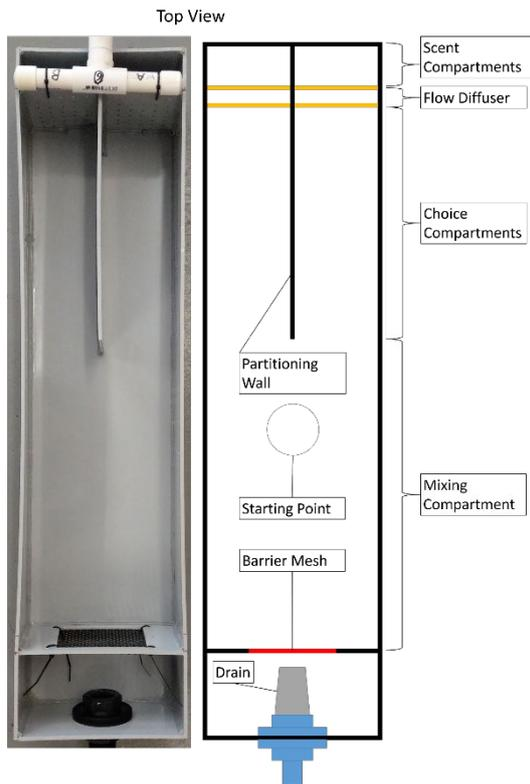
**Figure 44** Top view of the Y-maze showing the various components including the scent compartments, choice compartments and the starting location.
