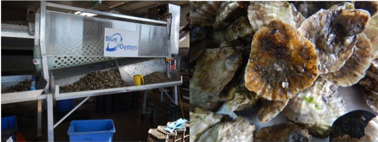
Figure 3.18 Rotating barrel grader selecting for 35 mm hole size grade (largest pile in photo) Native Oysters ( Ostrea angasi ) for grow-out trials in Blackman Bay, Dunalley, Tasmania, Australia.
