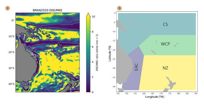
Figure 1 – a) Ratio of EKE to MKE and b) Four key regions defined for analysis. EAC = East Australian Current-dominated; CS = Coral Sea and Equatorial; WCP = Western-Central Pacific; and NZ = New Zealand.
