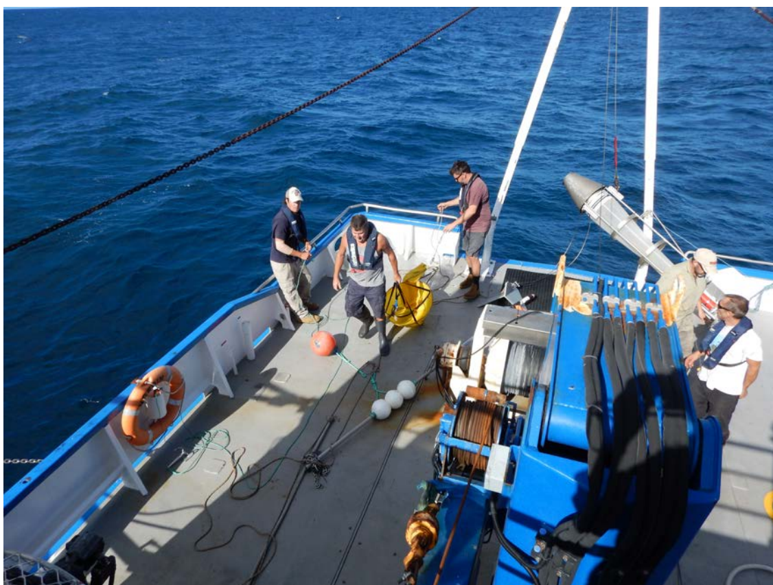
Figure 1. The drogue and buoy used to follow patches of eggs.
