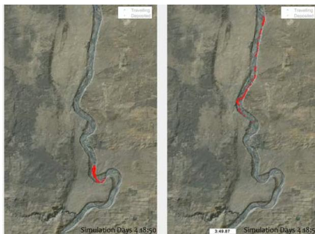
Figure 16b: Example output from the DCP model showing carp particle transport after input at two discrete locations in the lower River Murray domain.
