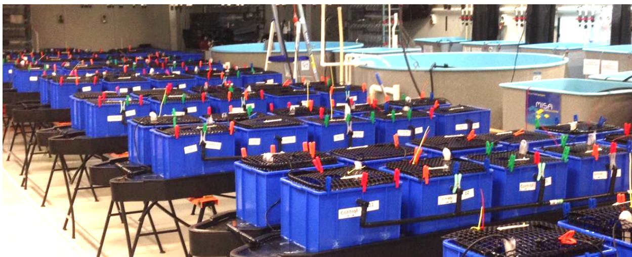
Figure 17.1 Biosecure experimental facility where lobster housed in individual tanks were exposed to PST through either food or toxic algal cultures.
