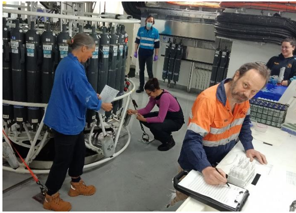
Figure 5.61 Water sampling from the CTD rosette.
