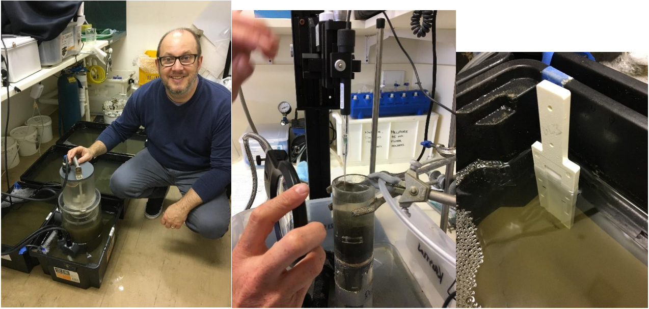
Figure 5.47 Sediment resuspension annular flume (left), oxygen microelectrode (centre), gel sampler for sampling porewater nutrient gradients (right).
