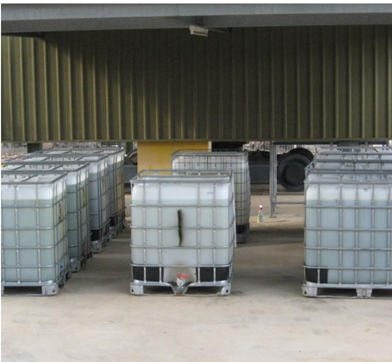
Figure 2: Carp concentrate production in IBCs at River Murray Lock 1
