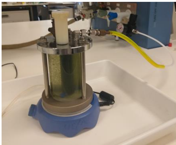
Figure 8: Stirred cell reactor for direct filtration simulation with 0.5 kg/m 3 carp density (alum + PAC treatment)
