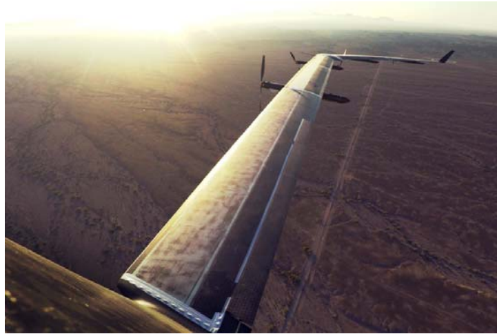
Figure 45. The Aquila high altitude drone, destined to provide internet coverage to remote regions during its maiden test flight in 2016 (Source: Facebook).
