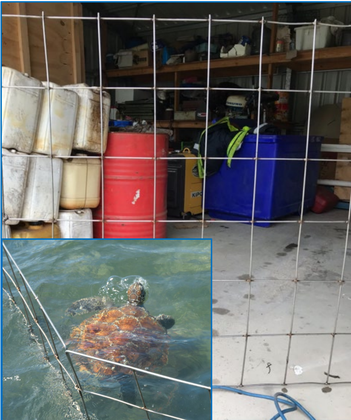
Figure 10: the exclusion grid is designed to keep larger animals such as turtles (inset) out of the tunnel. However, the dimensions of the grid used during the trials may have been too small to allow the primary target species (Barramundi and King Threadfin) to enter the tunnel. Note: inset photo was taken in Moreton Bay, no turtles were encountered during the field trial in Cardwell.
