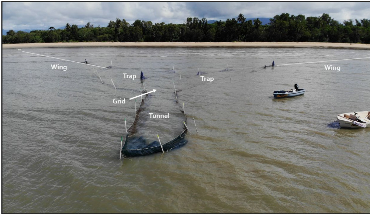
Figure 7: aerial view of a tunnel net deployed during the field trials showing the various elements of the gear.
