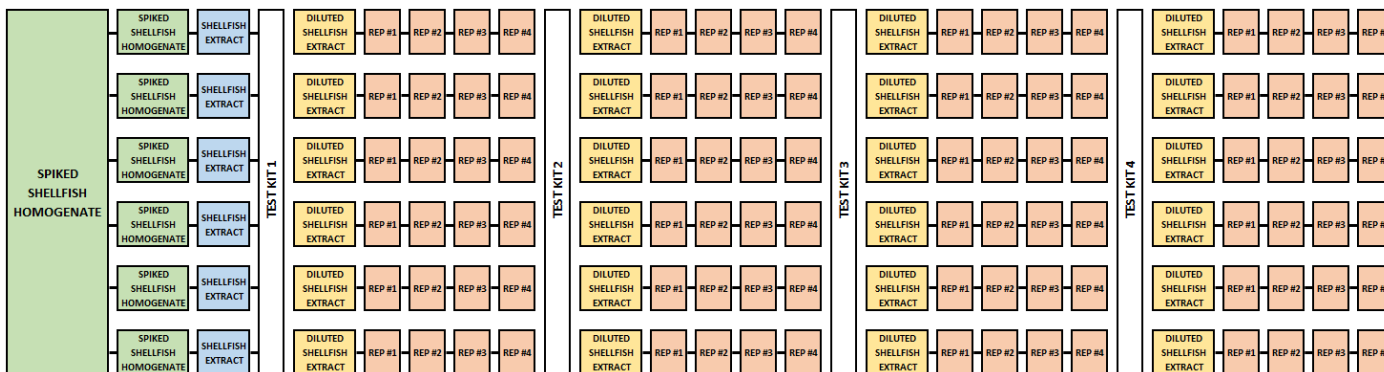
Figure 5: Experimental Setup used for Test #4. Six 1 g samples of the spiked shellfish homogenate were used to prepare six replicate shellfish extracts (and subsequently diluted shellfish extracts). Four replicate tests were conducted on each of the diluted shellfish extracts – this was repeated across 4 separate test kits.
