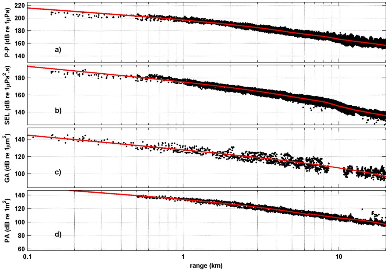
Figure 4. All measurements made of: a) peak-peak pressure; b) sound exposure level (SEL); c) the maximum magnitude of the 3-axis ground acceleration vector across an air gun signal; and d) the maximum magnitude of the 3-axis particle acceleration vector across an air gun signal. The red curves are fitted to each data set and were used for estimating exposures (see text).
