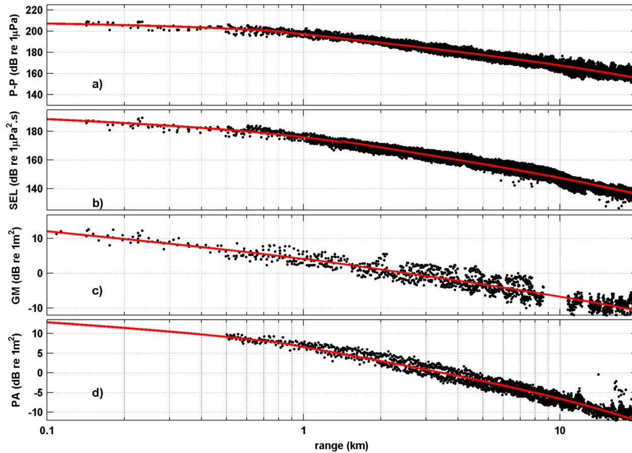
Figure 5. Received air gun levels in decibels with logarithmic slant range (black dots) showing: a) peak to peak; b) sound exposure; c) maximum magnitude of ground acceleration; and d) maximum magnitude of water particle acceleration. The red lines are fitted curves to the data.
