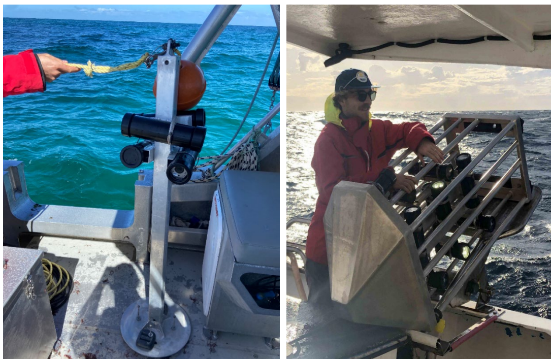
Figure 5 Lighter weight mono-configuration wide-field drop camera system being deployed by hand (left) and stereo-configuration wide-field drop camera system deployed from a commercial fishing vessel fitted with a 'pot tipper' (right).
