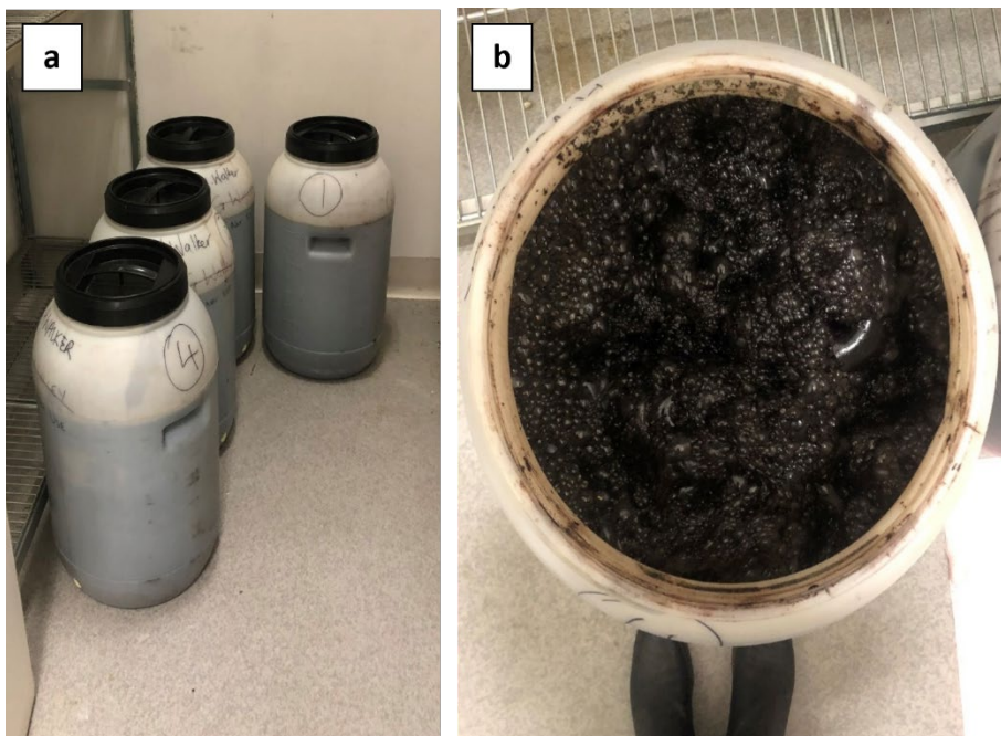
Figure 3. Liquid Sea Urchin waste (SUW) in barrels a) prepared for fermentation, b) SUW visibly fermenting
