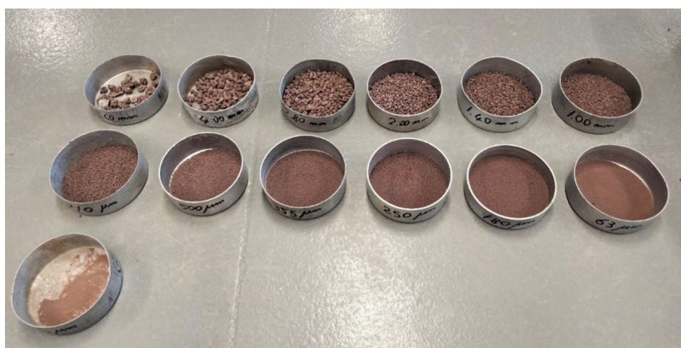
Figure 4. Separation of particle sizes from Sea Urchin waste product sample via particle size analysis
