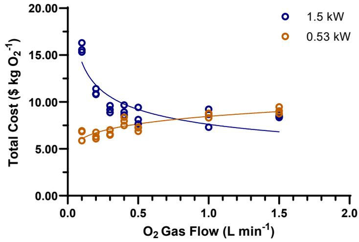
**Figure 13.** Total cost (pumping (kWh) + O<sub>2</sub> gas cost (transferred + lost) to transfer 1 kg DO into freshwater using two different wattage pumps. Nexus = 0.78 L min<sup>-1</sup>. Data shown for values established in 500 L aquaculture tanks.
