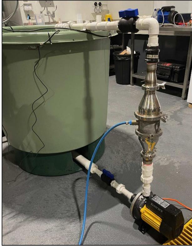
**Figure 9.** 500 L tank setup with NB injector and O<sub>2</sub> gas line attached, and 0.53 kW pump.
