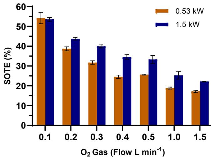
**Figure 11.** Standard oxygen transfer efficiencies ( $\pm$ SEM; n=3) for different capacity pumps and O<sub>2</sub> flow rates
