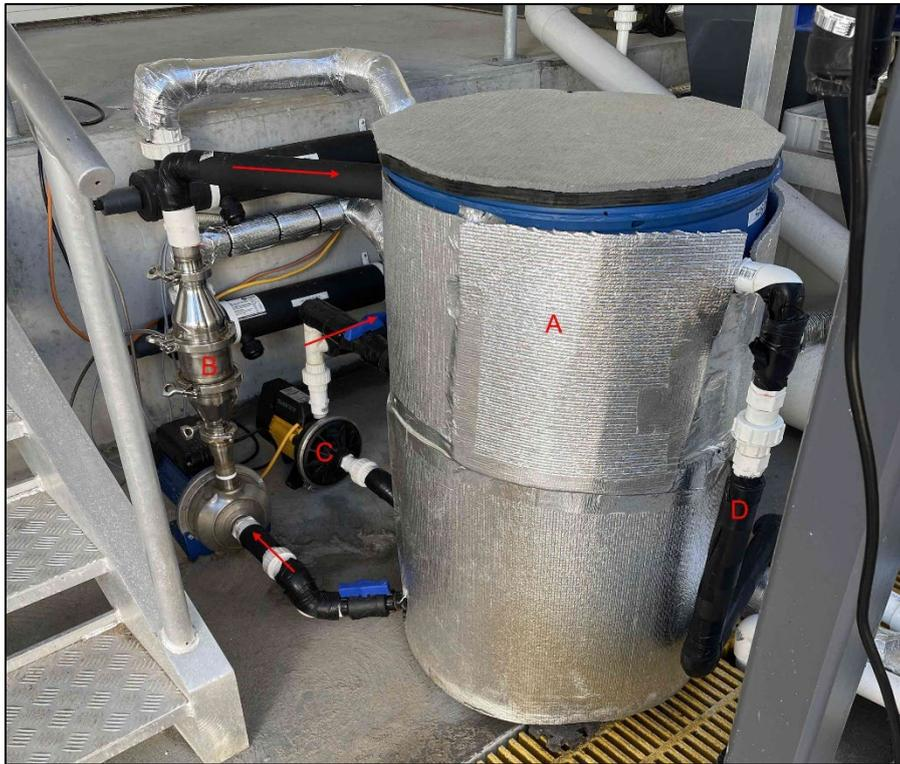
**Figure 1.** Configuration of NB injected saturation tank. Arrows indicate direction of water flow. A) 200 L saturation tank, B) NB injector, C) RAS and experiment tanks supply pump of NB saturated water, D) water top-up recirculation line from RAS.
