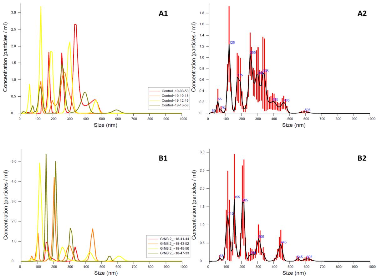
**Figure 15.** Nanobubble concentration and size in saltwater control (A) and nanobubble (B) treatments. (1) Finite track length adjustment (FTLA) Concentration/Size ( $n=4$  runs), and (2) averaged FTLA Concentration/Size. Error bars indicate  $\pm 1$  SEM.
