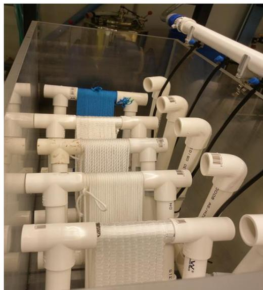
**Figure 14:** Airlift Suspension Technology (AST) prototype developed at DPI-NSW for protoplast seeding and germination.
