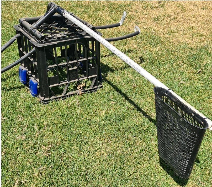
Figure 1. Portable baited video setup used from the shore during the project.
