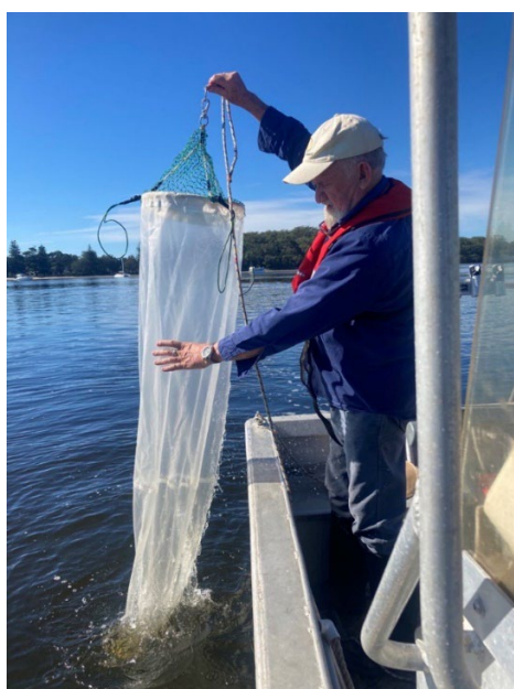
Figure 2: Plankton net with 100 µm mesh used for zooplankton sampling.
