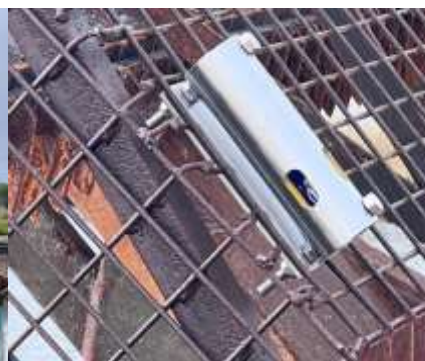
Final placement of sensor and Stainless Steel casing on dredge
