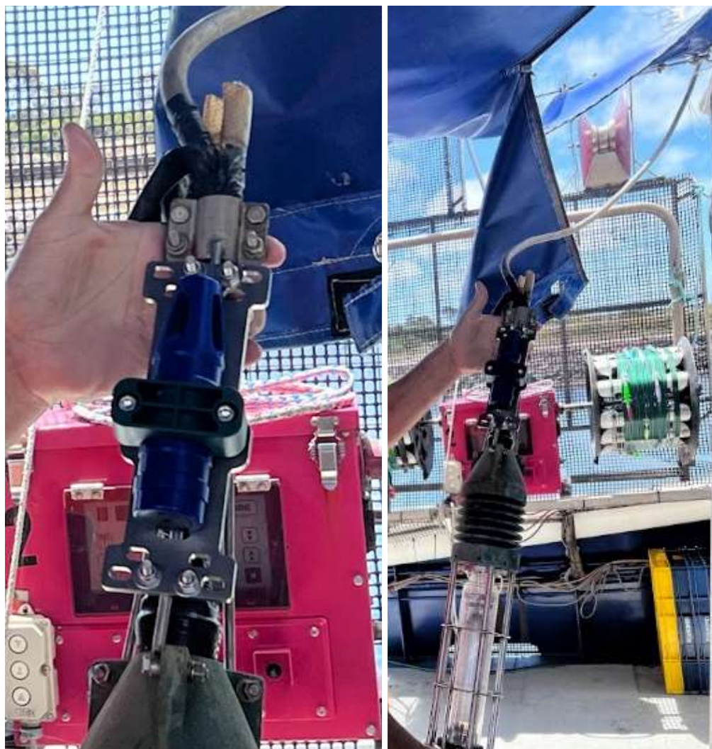
Figure 5 Placement of a sensor on the reinforced cable attached to the deepwater light on a squid jig vessel.
