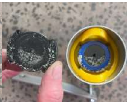
Sensor and casing filled with sand and shells
