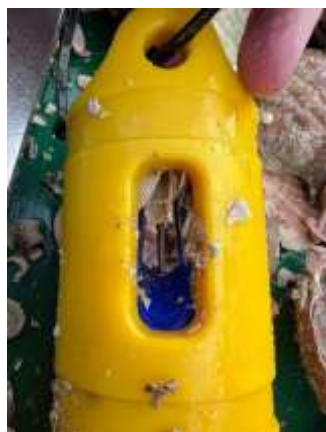
Sand and shell grit filling the sensor casing openings
