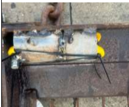
Trial casing to protect sensor impeded water flow
