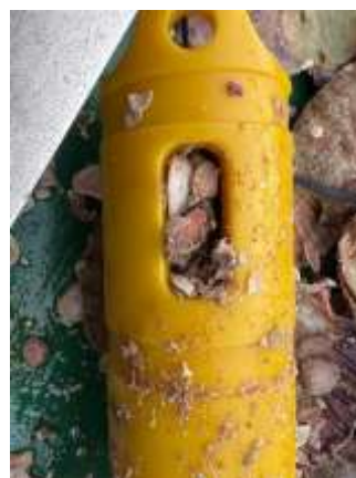
Sand and shell grit filling the sensor casing openings
