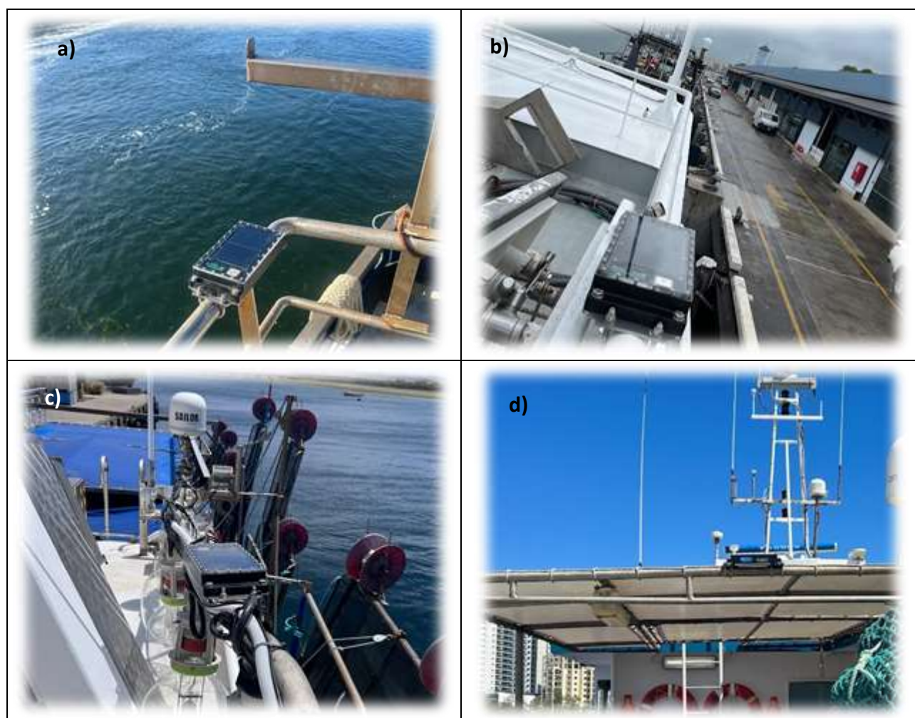
Figure 2. Various installations of deck boxes on commercial fishing vessels: a) scallop dredge vessel, b) prawn trawler, c) squid jig vessel, d) fish trawler.
