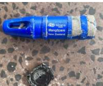
Sensor and casing filled with sand and shells
