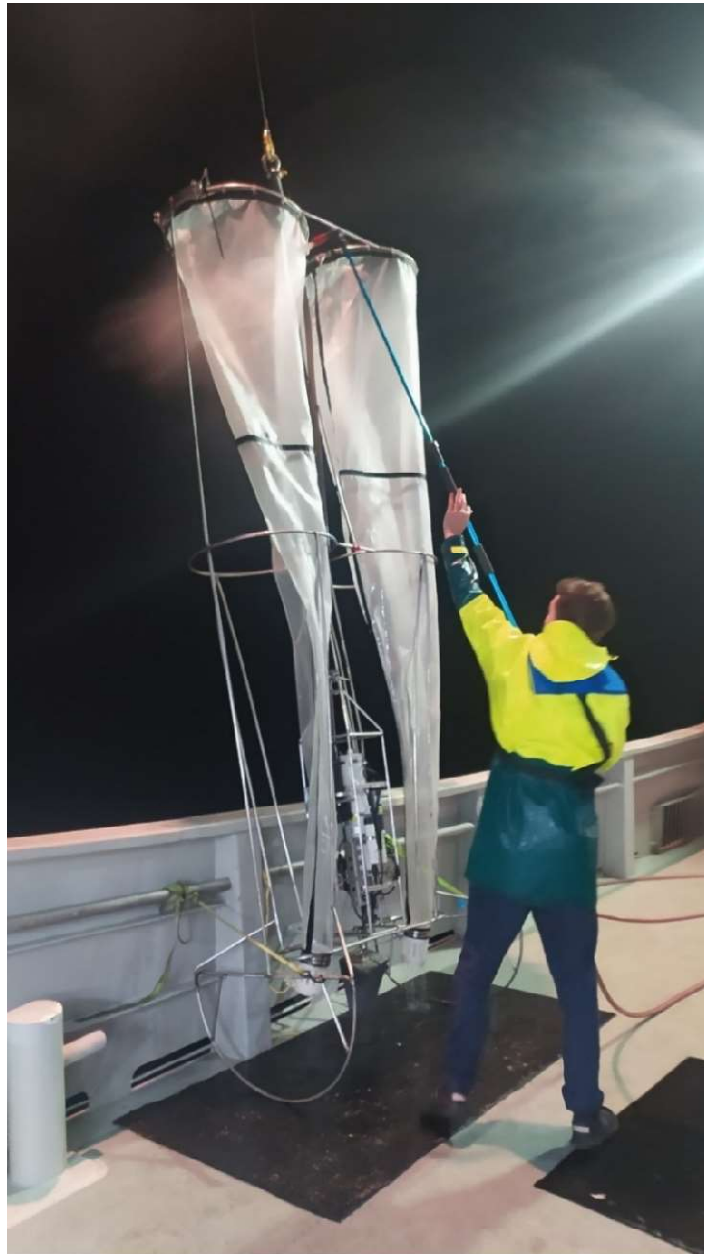
Figure 4. Photograph of the sampling device with paired bongo net and CTD deployed during the survey.
